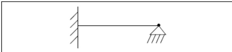
Figure 8 Beam with Fixed-Pinned Boundary Conditions
